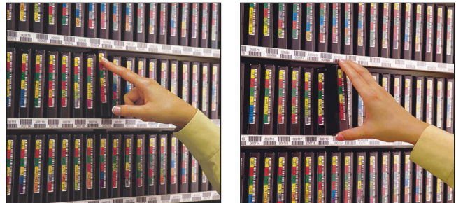
Spring ejection assists in fast tape retrieval.
